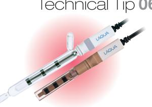
onductivity cells, also called conductivity electrodes or probes, are constructed with metal electrodes placed ✓at a fixed distance in either glass or plastic body and surrounded by an outer tube. The distance between the electrodes divided by their surface area is known as cell constant. HORIBA offers two-electrode conductivity cells with cell constants expressed in cm<sup>-1</sup> and m<sup>-1</sup> units.
